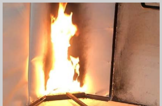
↑ A2-s1,d0 fire shaft burntest proves the non-flammable properties
