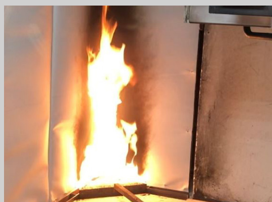
↑ A2-s1,d0 fire shaft burntest proofs the non-flammable properties
